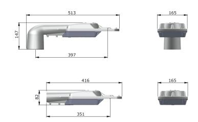
\*Nominal pole/bracket diameter shown Tolerance ±2mm allowed
