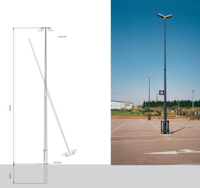
14m mid hinge octagonal steel column with plate to fit floodlight bracket. Maximum weight of bracket and floodlights 70kg. Column has large base for control gear or large fuse cut-out. Base compartment can be accessed without lowering the column. Finish hot dip galvanised. Column is supplied in component form for assembly on site.
