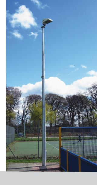
12m mid hinge octagonal steel column with plate to fit floodlight bracket. Maximum weight of bracket and floodlights 44kg. Column has large base for control gear or large fuse cut-out. Base compartment can be accessed without lowering the column. Finish hot dip galvanised.
